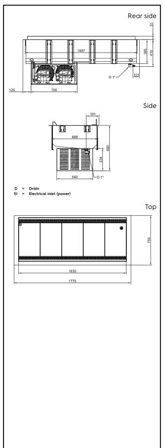
$\qquad \qquad \text{Drop-In} \\ \text{Drop-in refrigerated well, ventilated (5 GN container capacity)}$
