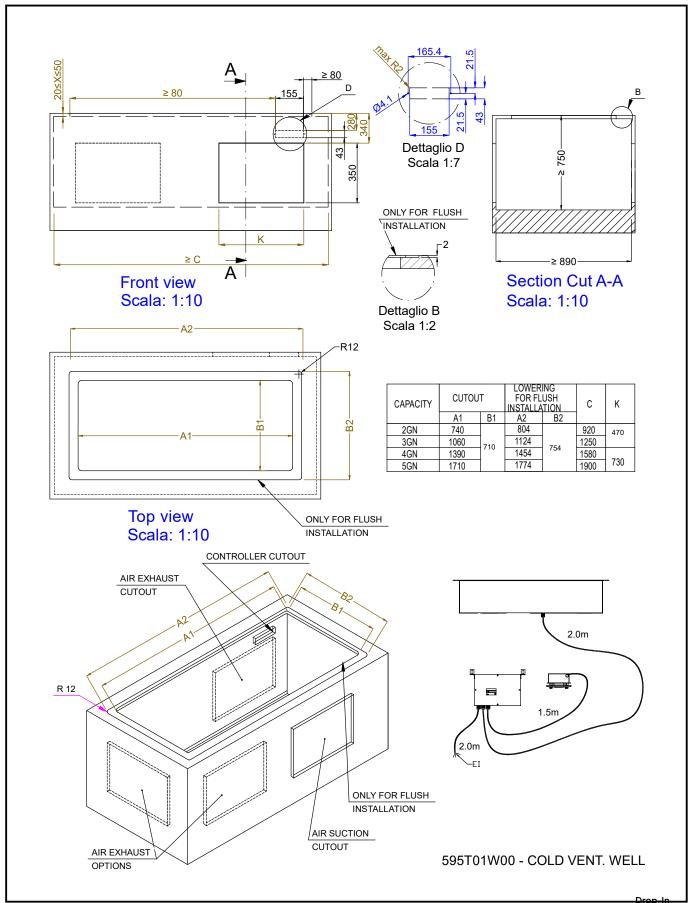
Drop-in refrigerated well, ventilated (5 GN container capacity)
